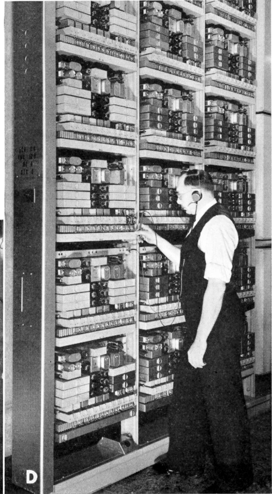
Fig. 2B—Two sender-link controllers and their connectors comprise the bay at the right. The primary and secondary switches of a sender-link frame occupy two bays, as shown at the left of the controllers
